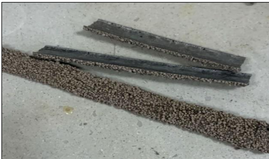
Picture 2: A metal-containing hot layer formed on the weld as a result of electrode welding
