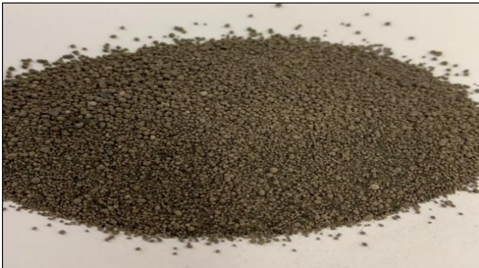
Picture 1: Waste in the form of metal-containing dust generated on the weld as a result of electrode welding
