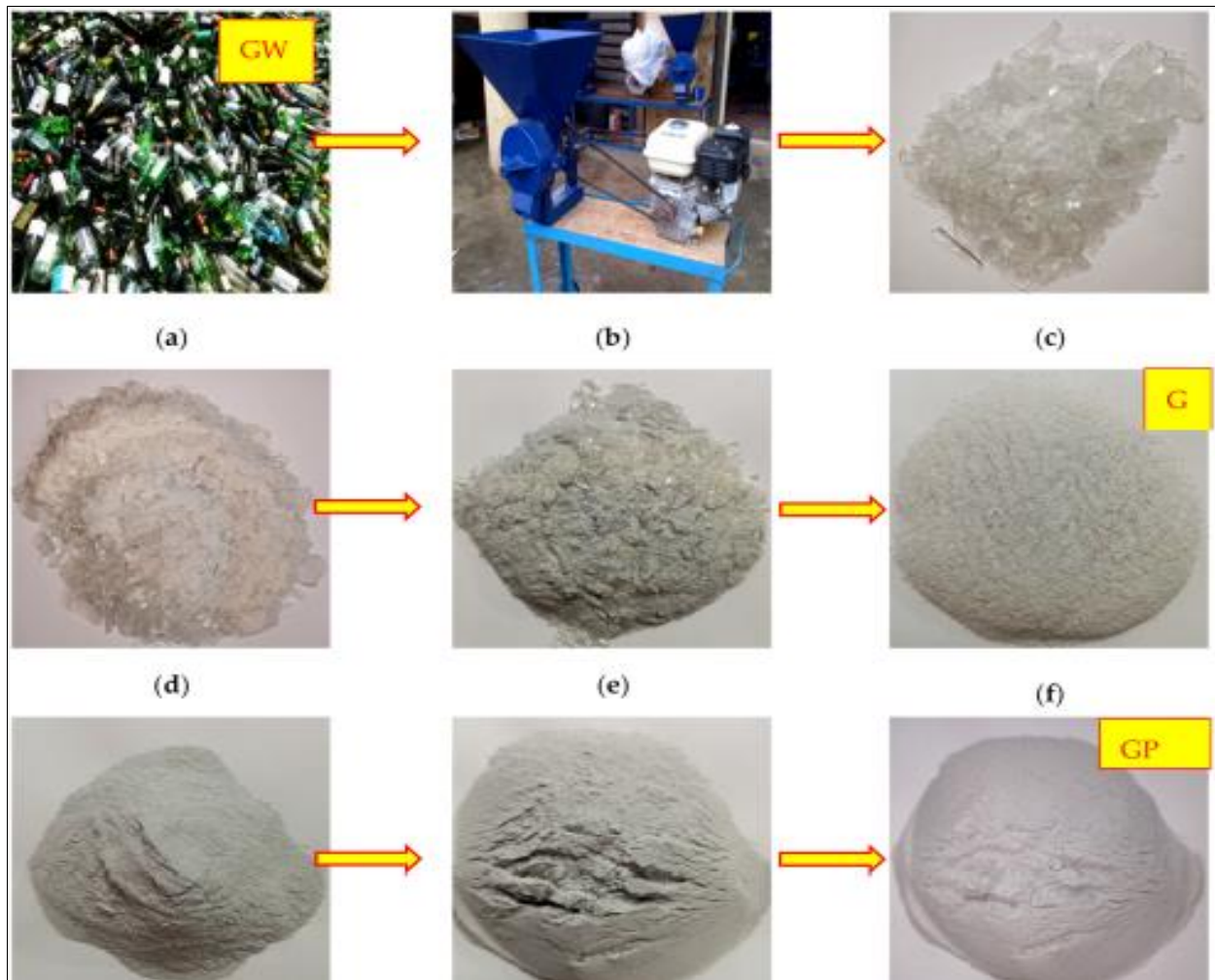
Fig 3: Different stages for glass waste milling. (a) Glass waste (GW); (b) ground mill; (c) crushed glass (size \gg 4.75 mm); (d) crushed glass (size \gg 4.75 mm); (e) crushed glass (size > 4.75 mm); (f) glass particles (G) used as fine aggregate (size < 4.75 mm); (g) milled Glass (size \ll 4.75 mm); (h) milled glass (size \ll\ll 4.75 mm); and (i) glass powder (GP) used as a substitute for PC (size < 75 \mu m).
