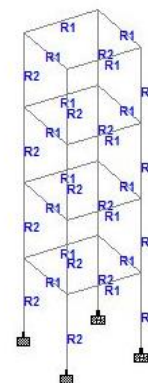
Fig 6: skeletal structure without damper MDOF
