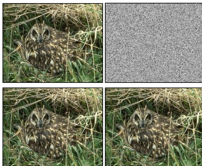
Fig 5(a) (b) (c) (d): Results demonstration of proposed method with ER 1.33 bits per second. (a) Original image. (b) Encrypted image. (c) Directly decrypted image (d) Reconstructed image.
