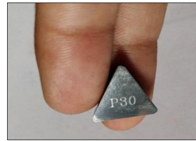
Fig 2: Coated carbide Insert (P30)
