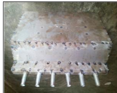
Fig 7a: Fabricated Hopper setup with hole arrangements at bottom side
