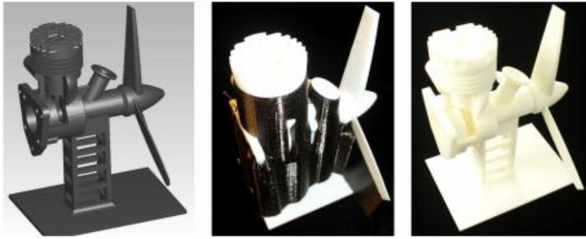
Fig 4: (a) Original STL (b) prototype with support material (c) prototype without support material
